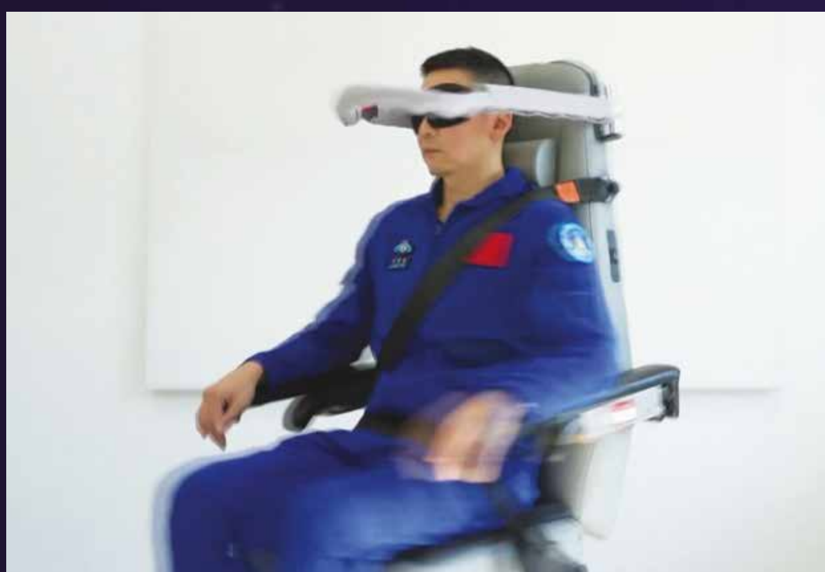
航天員在轉椅上快速旋轉，以訓練內耳能力，減輕進入失重環境時出現眩暈 Astronauts spinning in high speed to train their inner ear function, helping reduce dizziness when entering a weightless environment
